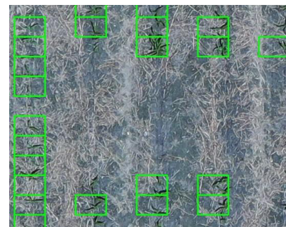
Figure 4. Example of a corn counting model output. The counter module will draw bounding boxes only around the corn plants.
